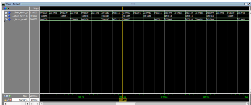
Figure 6.a: ModelSim of VHDL Code for Bitwise AND
