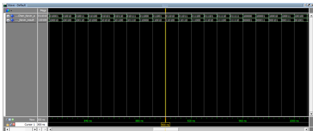
Figure 12.b: ModelSim of VHDL Code for Rotation Left
