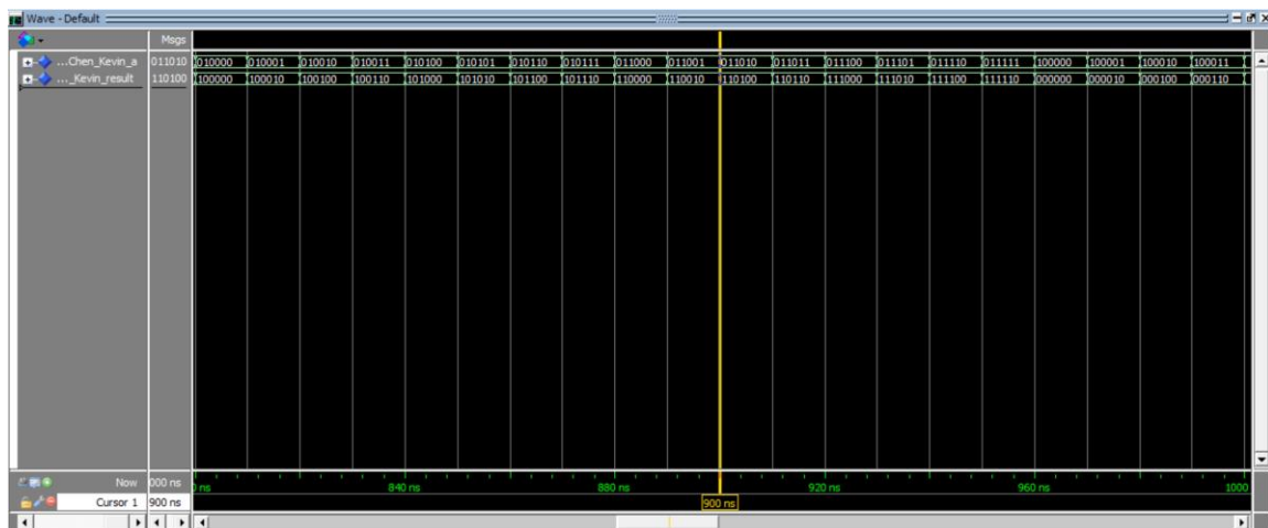
Figure 10.b: ModelSim of VHDL Code for Shift Left
