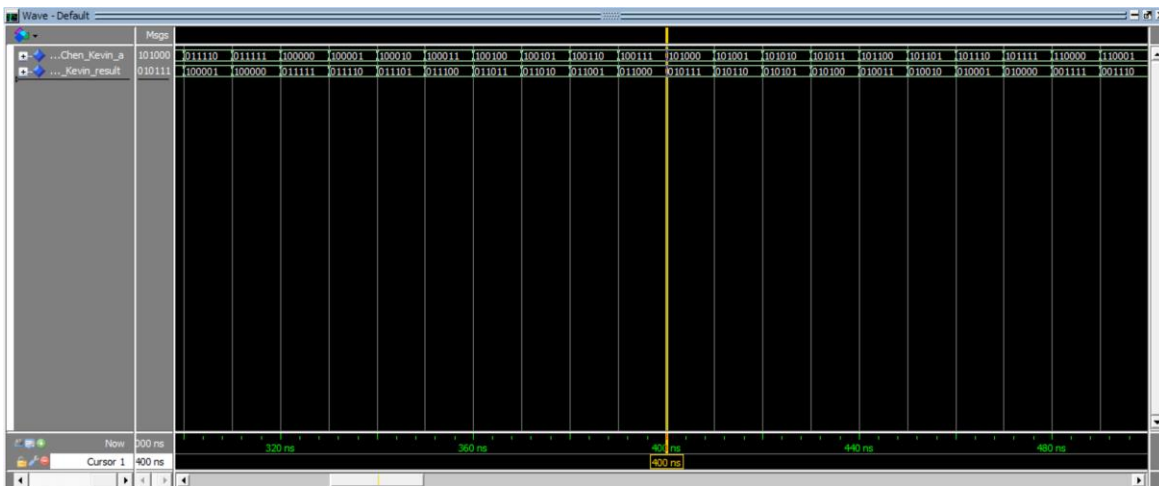
Figure 9.a: ModelSim of VHDL Code for Bitwise NOT
