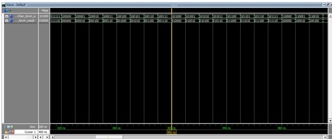
Figure 10.a: ModelSim of VHDL Code for Shift Left
