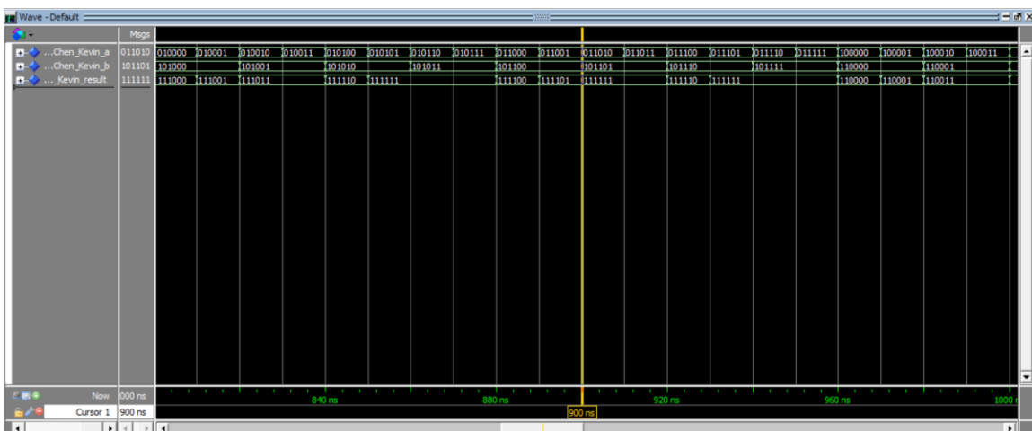
Figure 7.b: ModelSim of VHDL Code for Bitwise OR
