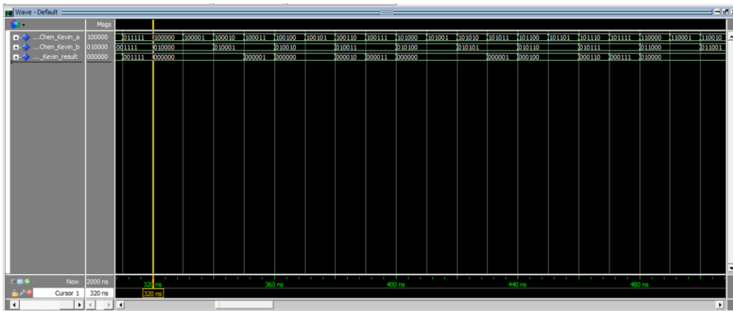
Figure 6.a: ModelSim of VHDL Code for Bitwise AND
