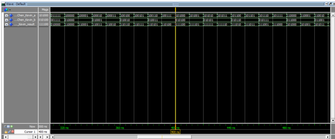
Figure 8.a: ModelSim of VHDL Code for Bitwise XOR
