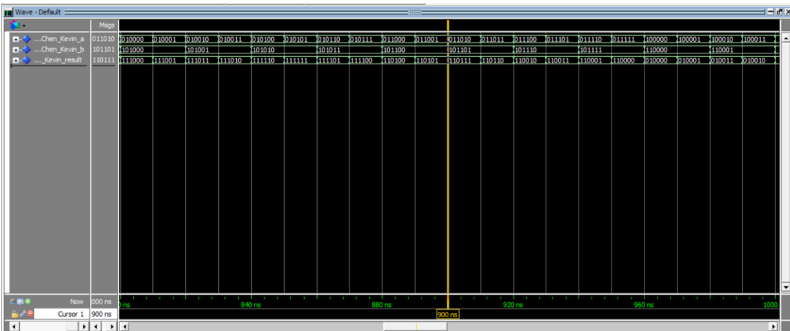
Figure 8.b: ModelSim of VHDL Code for Bitwise XOR
