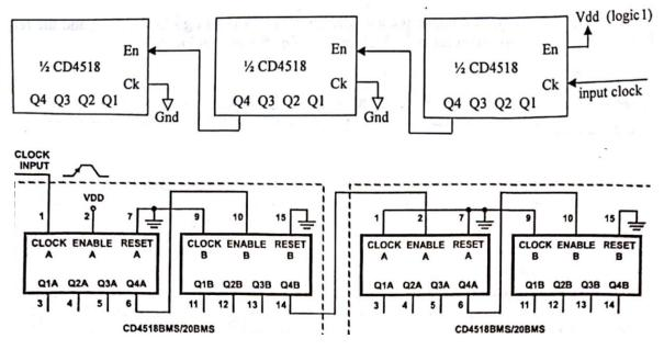
The design for the connection between the CMOS IC are shown below:
