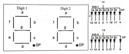
There is a total of 18 pins. Pins 13 and 14 should both be connected to the power source to supply all the segments power. You can make a certain segment light up by connecting the ground to any of the other pins.
