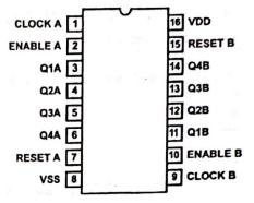
There is a total of 16 pins. This CMOS IC is specifically for the minutes/seconds counter of the clock. We're going to need two of these, one for each two digits. We start off by connecting pin 16,  $V_{DD}$ , to the power source to make sure power is supplied. We connect pin 8,  $V_{SS}$ , to ground. We then connect pins 3, 4, 5, 6, the Q's, each to the corresponding BCD inputs on the CD4543BE CMOS IC. We do the same for pins 11, 12, 13, and 14, the Q's.
