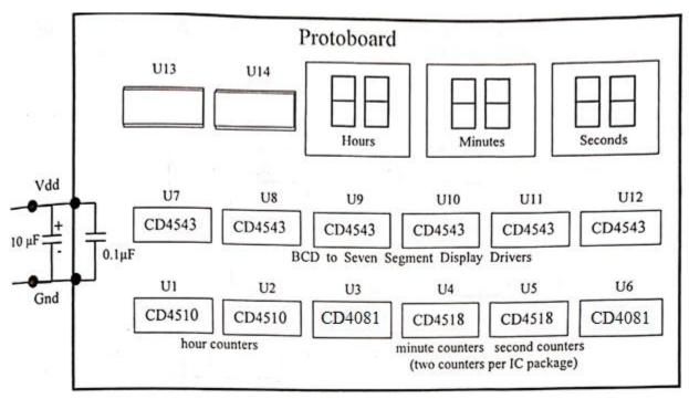
NOTE: The pin assignments of any circuit part are counted from the bottom left to the bottom right to the top left in numerical sequence.
