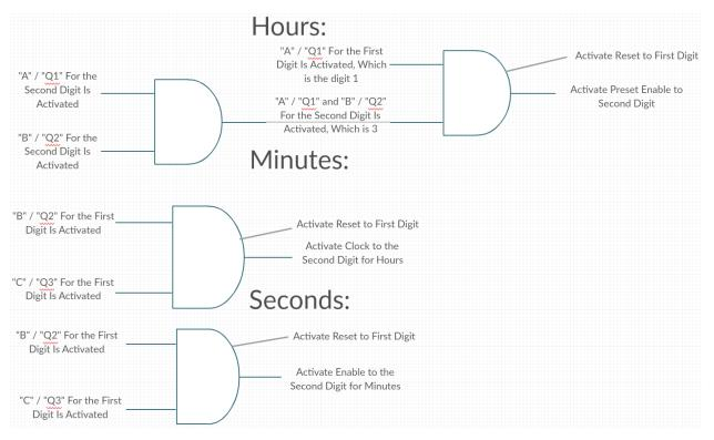
After knowing how the logic of the clock works, just connecting the wires to it's appropriate location and turning on the DC power supply and function generator would allow the 12-hour digital clock to start working. Make sure the DC power supply supplies at least 5 V. In addition, the settings for the function generator should be in a square wave, with a frequency of 1 Hz, for it to count in seconds, and having a maximum of 5 V and a minimum of 0 V.
