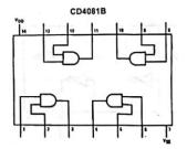
There is a total of 14 pins. We start off by connecting pin 16,  $V_{DD}$ , to the power source to make sure power is supplied. We connect pin 8,  $V_{SS}$ , to ground. Pins 1, 2, 5, 6, 8, 9, 12, and 13, inputs, all work the same way. They take the input and logically display an output. The outputs are pins 3, 4, 10, and 11. The output will only be 1 if both inputs are 1. This is important for the logical for the resets.
