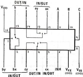
It uses a triple 2-channel analog multiplexer and the truth table is shown below. Its purpose is to set the time for the hours, minutes and seconds by increasing its increment when the button is pressed.
