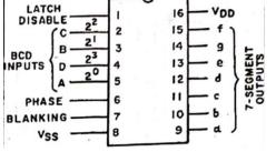
There is a total of 16 pins. We connect pin 9-15 to the corresponding 7-segments, making sure each letter is connected to each other. We connect pin 16,  $V_{DD}$ , to the power source and pin 8,  $V_{ss}$ , to the ground. In addition, we also connect pin 1 and 6, Latch Disable and Phase, to the power source, and pin 7, Blanking, to ground.
